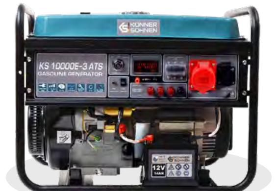
\* KS 10000E series models (single-phase) have the possibility of welding inverter connection with maximum current up to 200 A, only in case that the welding inverter has 85% efficiency and an arc voltage of 25 V.
