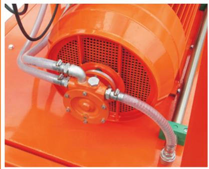
Built in mechanical feed pump.
