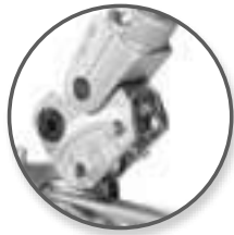
Roller Dies Reduce Force and Tube Flattening
