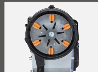
Grinding width 170 and 250 mm
