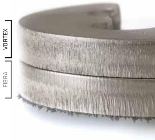
Cutting comparison on 10mm stainless steel between a 4kW fiber laser system with and without Vortex cutting process.
