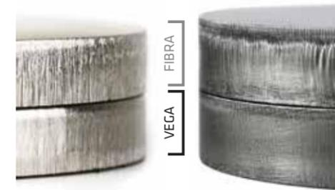
Cutting comparison on 10mm stainless steel (left) and 15mm carbon steel (right) with and without Vega cutting process.
