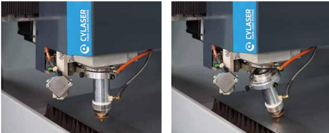
Example of collision check system function
