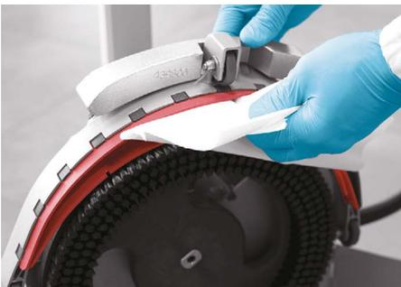
To ensure a perfect drying, the suction hose and the squeegee rubber blades must be cleaned at the end of any cleaning operation. The squeegee can be lifted to quickly clean the rubber blades
