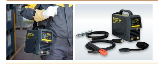
160 200 +10% -10% Single phase input 50/60 Hz V 230 230 Input Power @ I, Max 9,2 10,4 kVA 16 Delayed Fuse (I eff) 16 А Power Factor /  $\cos \phi$ 0,67/0,99 0,67/0,99 Efficiency Degree 0,82 0,81 Open circuit voltage 72 72 V 10 - 200 10 - 160 Current range А 95 105 100% А Duty cycle at (40°C) 60% 105 110 A Х% 160 (20%) 200 (10%) A EN 60974-1 • EN 60974-10 Standards S **Protection Class** IP 23 S 23 S **⊅** mm 315 315
