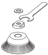
Steel wire brush Ø 115 mm
