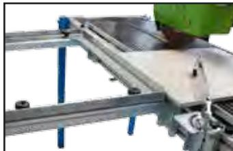
Side support with two clamps, improves precision while cutting (optional).
