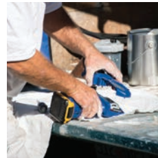
2. Remove the old pump from the sprayer.
