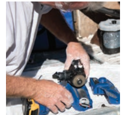
3. Place the new pump into sprayer.
