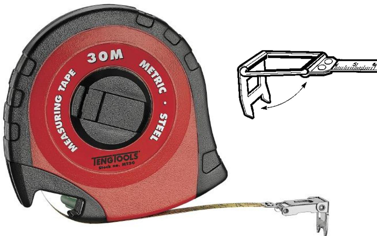
**Teng Tools** Steel measuring tape with nylon coating and anti-reflection surface. 10 mm tape width. Graduated in mm and inch. High impact plastic case with rubber grips on the sides. True zero hook for internal and external measurement.
