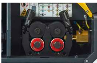
Professional double groove feeding mechanism with 4 rolls
