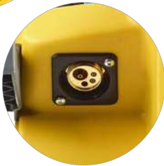
INCLINED TORCH CONNECTION
