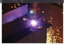
**Connected bolt hole** cutting and combining cut sequences to save on time and ignitions enable a significantly shorter throughput time while extending consumable life time. Practically eliminate grinding
