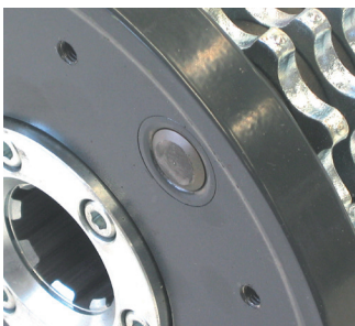
Drum with replacement bushes = longer service life
