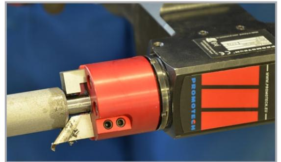
Extension set for pipes from ID 42 mm (1.65")
