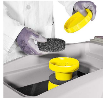
For an effective vacuuming the suction filter must be kept clean
