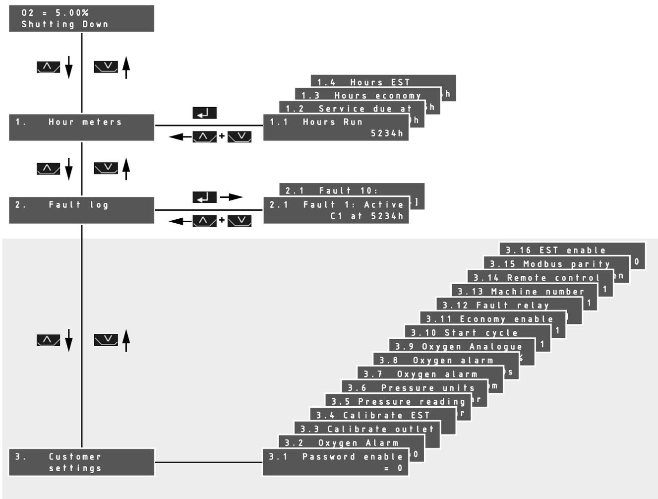
The interface will automatically default back to the main operating menu if no key activity has been detected for one minute.
