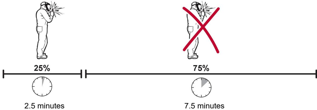
A different combination of duty cycle and welding current can be selected. Use the graphs below to determine the correct duty cycle for a given welding current.
