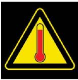
The welding power source has overheating protection that operates if the internal temperature becomes too high. When this occurs, the welding current is interrupted and an overheating symbol appears on the display. The overheating protection resets automatically when the temperature has returned to normal working temperature.
