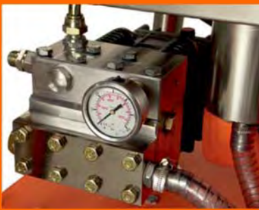
Stainless steel pump-head. Integrated unloader valve.
