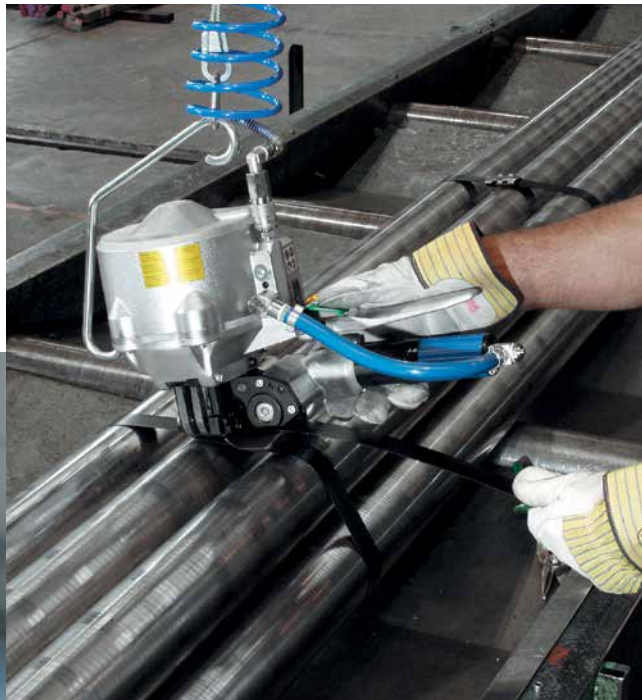
Manual tensioning and sealing
