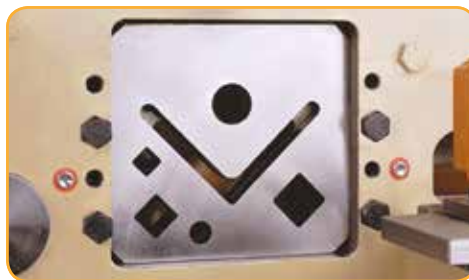
\emptyset and \square cut without deformation
