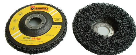
Discs made of a nylon threads mesh bonded with resin to abrasive. It is for the mechanical pickling of all kinds of weld bead and for the removal of paints, saltiness, rust and grease.
