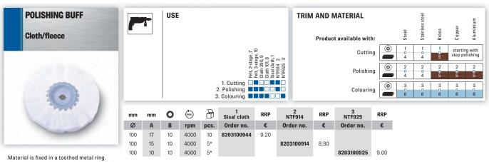
Material is fixed in a toothed metal ring. The polishing buff is clamped using conical spring washers.
