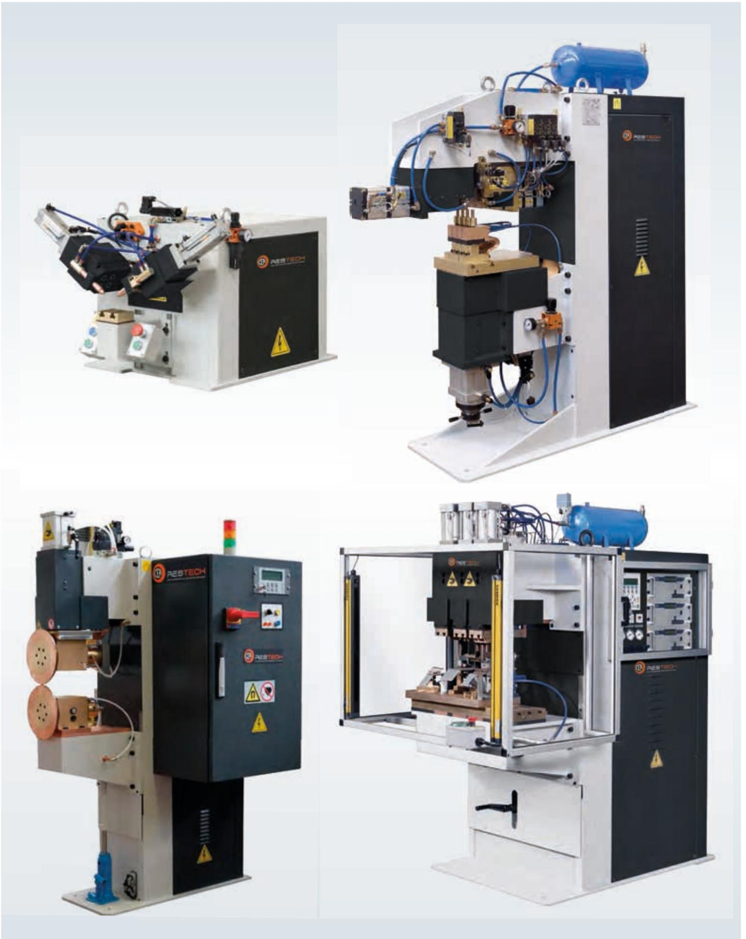
CEA RESTECH new catalogue offers a complete range of electronic controls and component kits suitable for integrators, special machine manufacturers and also for any retrofit job to upgrade any old generation resistance equipment. The resistance specialists will be able to find a really large variety of components for single phase, three phase and latest generation inverter based technologies with related electronic controls, power panels and transformers able to fully meet any industrial needs.
