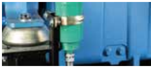
Heavy-duty anti-vibrations mountings
