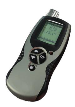
The DPM-120 is a multi-functional instrument which can be used to measure, record, and analise the important climatic parameters in the surface treatment of metal substrates: air temperature, surface temperature, relative humidity, dew point. Additional information such as the time and date of readings taken are recorded for future reference. The ergonomic and tough DMP-120 is supplied in a convenient protective carry case.
