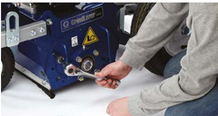
1. Loosen four bolts
