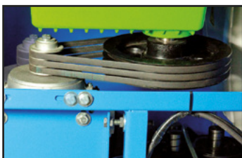
New easy and quick belts tightening system.
