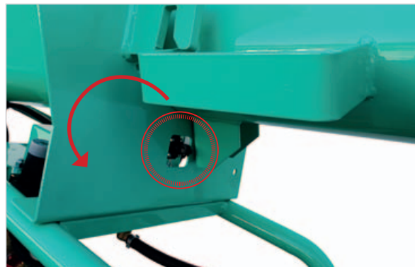
Safety sensor if the mixing chamber is opened
