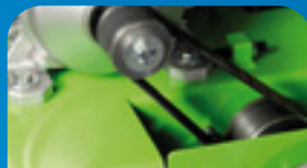
Poly-V belt transmission improves grip and reduces maintenance (BALI 500 MKN)
