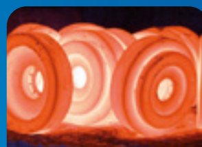
Inner components tempered for extended working life
