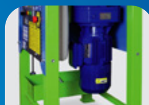
Heavy-duty motor-reducer, 0% power loss
