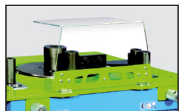
Curved protection visor for 360 degree visibility.
