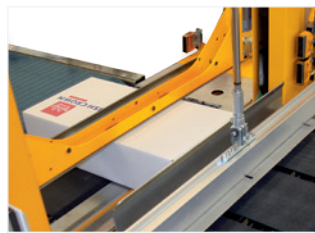
Package / bundle stop For positioning of loose bundles or packages
