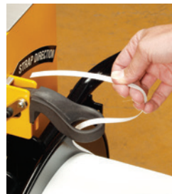
Simple strap coil change: minimum downtime time when changing the coil thanks to automatic threading
