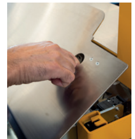
Optimum accessibility and tool-free maintenance
