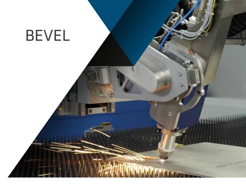
It is usually adopted to **increase the surface area of the edge for a stronger and consistent welding.** There are different types of bevelled edges which are indicated by the letter of the alphabet that mostly resembles the shape of the cut when seen in cross-section. The most common types of bevelled cuts include V, A, X, Y upwards, Y downward and K.
