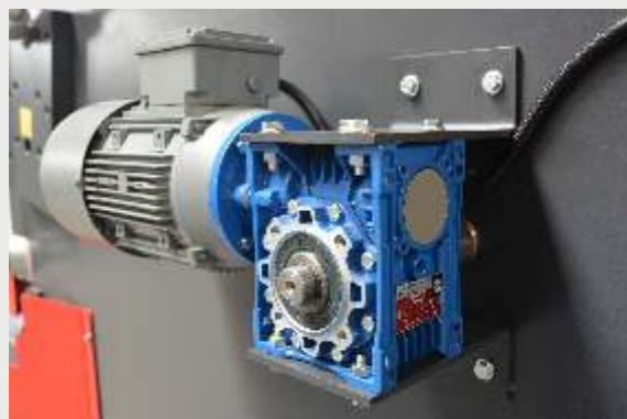
Motorized Blade Gap Adjustment with CNC Controller
