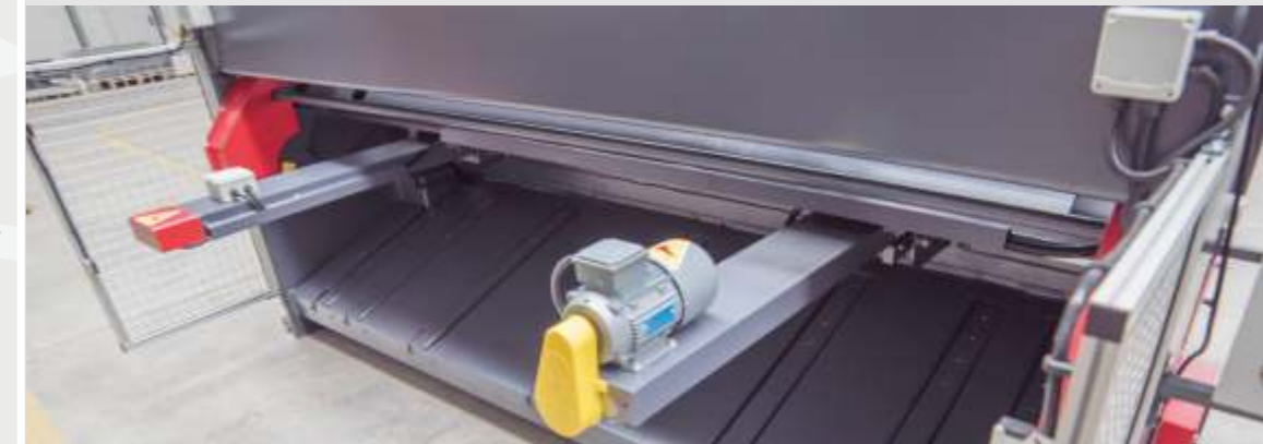
Motorized Back Gauge has \pm 0,1 mm Accuracy
