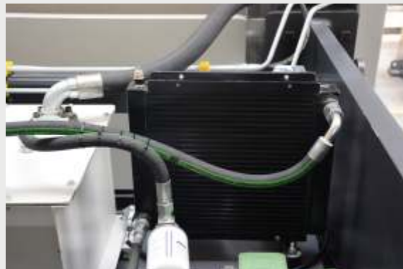
Hydraulic Oil Cooler System
