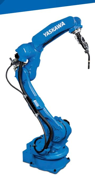
The powerful, dynamic six-axis MOTOMAN AR1730 robot provides highest motion performance in its class to achieve optimal results in extremely difficult conditions and especially for the high demands of arc welding applications.
