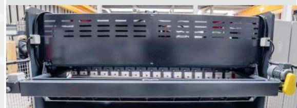
Motorized Back Gauge has \pm 0,1 mm Accuracy
