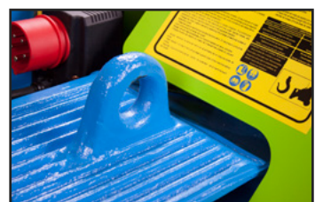
Lifting hook for easy transportation and shifting.
