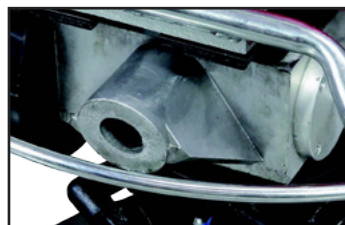
Slot for transportation bar.
