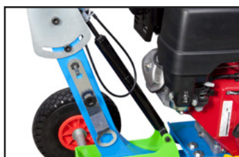
Cutting depth regulated by pneumatic gas shock absorber.
