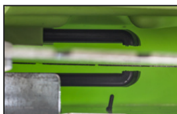
Water cooling fork, reaching both blade sides.
