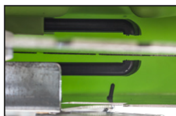
Cooling system for both blade sides.
