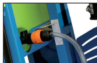
Cutting depth indicator.
