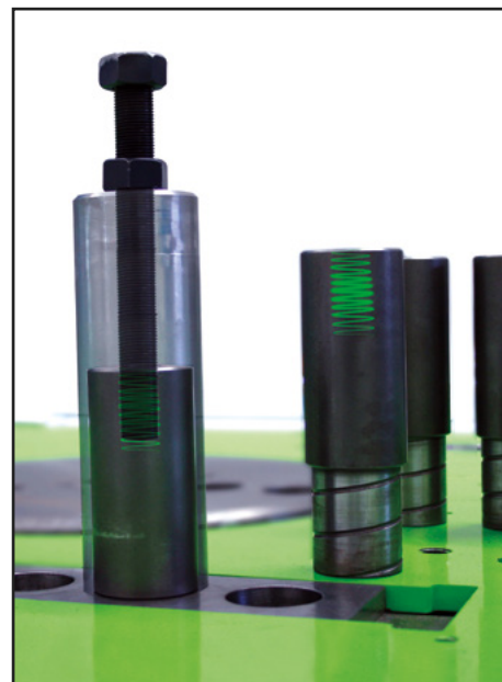
R202525006700. Pins extraction bolt.
