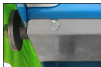
Protection guard for the gears and the blade shaft.
