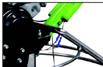
The triple tube arm is removable. Inside, the electric wiring and the accelerator.
