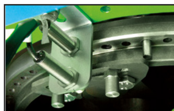
Dirt and water resistant IP65 inductive sensor.
