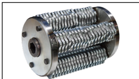
R971537000. Drum (mounting 80 milling cutters in four shafts) for CAT 202.
