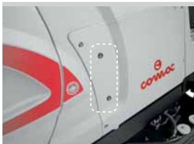
Fluid level indicator (version with CDS)
