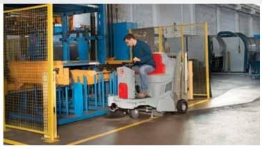
CS700/800 B-H are ride-on sweeping machines with automatic traction, powered by battery or gasoline motor, with a 70 or 80 cm working width (central brush).
