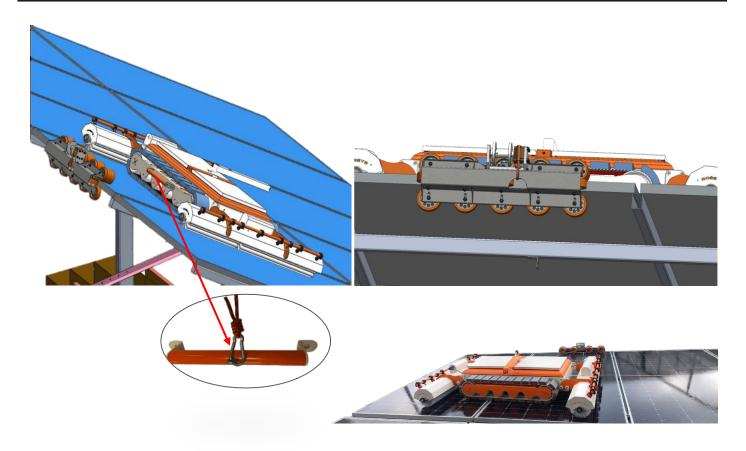
**Note:** The panel construction should not interfere with the movement of the suspension wheel.
