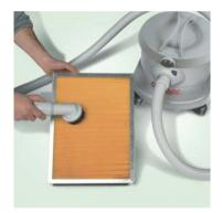
It is important to clean the panel filter with a vacuum cleaner after each cleaning task in order to guarantee perfect machine performance
