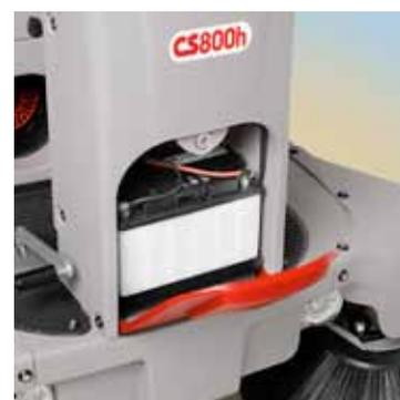
In the motor equipped versions (CS700-800 H), the start-up battery is located in the front compartment and can be easily accessed for inspection purposes.
