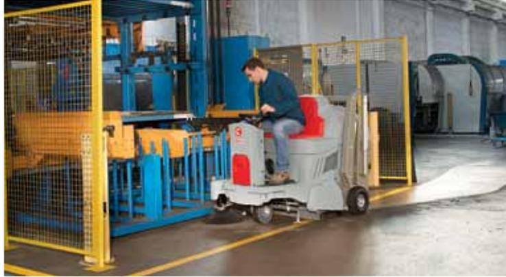
CS700/800 B-H are ride-on sweeping machines with automatic traction, powered by battery or gasoline motor, with a 70 or 80 cm working width (central brush).
