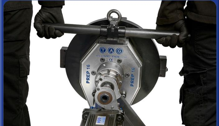
To enable ease of set up, the machine is equipped with lifting handles and removable extensions so the machine can be easily installed, and removed from the pipe.
