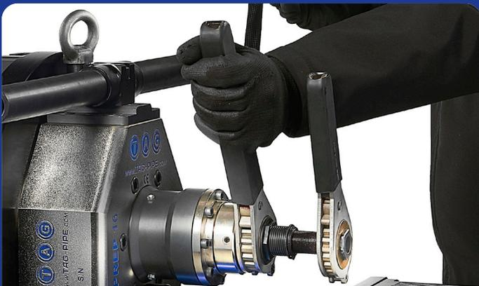
The PREP 16 has unrivalled power and stability, utilising a ratchet system for both jaw locking, and bevel feed.
