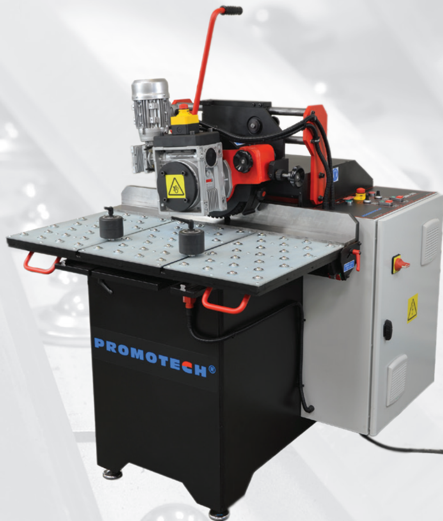
Pipe OD beveling from 50 mm up to 150 mm (option)
