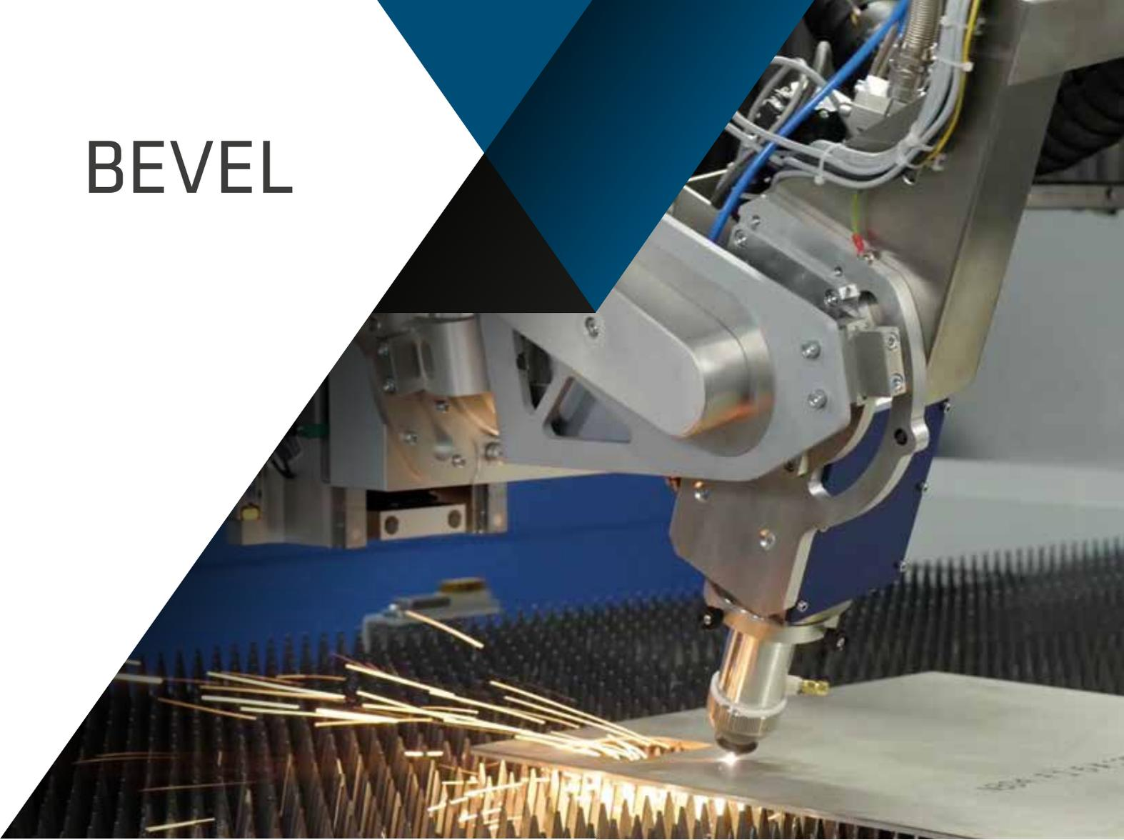
It is usually adopted to **increase the surface area of the edge for a stronger and consistent welding**. There are different types of bevelled edges which are indicated by the letter of the alphabet that mostly resembles the shape of the cut when seen in cross-section. The most common types of bevelled cuts include V, A, X, Y upwards, Y downward and K.
