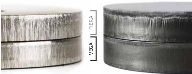
Cutting comparison on .400" stainless steel (left) and .600" carbon steel (right) with and without Vega feature
