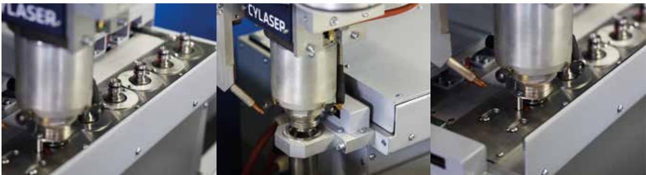
Thanks to the successful integration of the automatic nozzle changer device in its fiber laser cutting systems equipped with automation, Cy-Laser has decided to extend this option to the entire product range. With the possibility of choosing between **6, 12 and 18 nozzles formats**, the overall performance of the system definitely increases. As materials and thicknesses may vary throughout the
