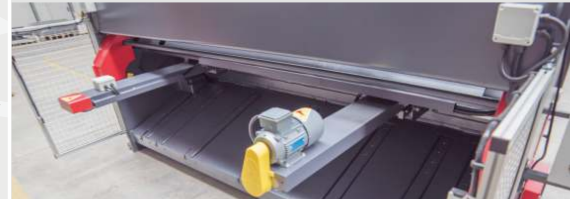
Motorized Back Gauge has \pm 0,1 mm Accuracy
