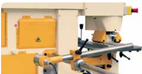
"Touch & Cut" Electric Length Stop 1 meter long
