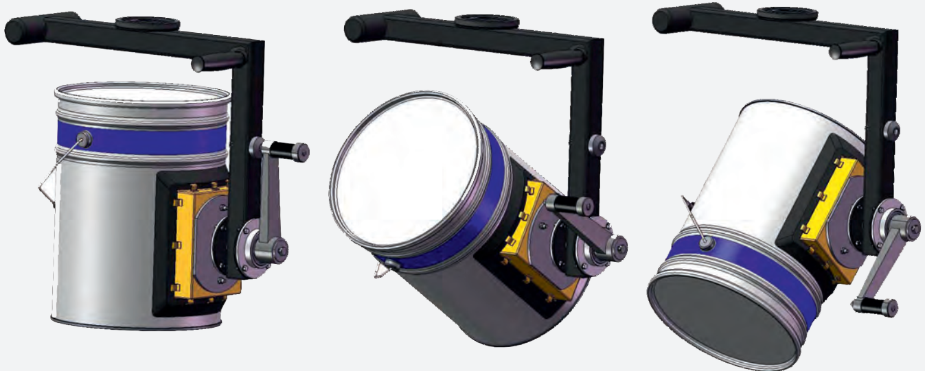
Kegs and tins need to be gripped from the side and rotated manually. Kegs because they are normally turned before storage and tins and pails (of paint) to secure the seal of the lid. Project nr 4558.
