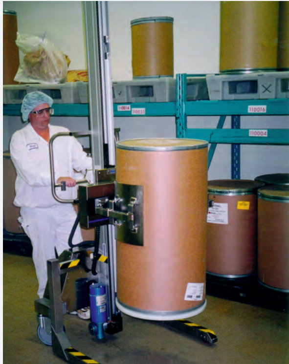
Heavy-duty PRO200ESE with grippers, max capacity 130 kg this version.
