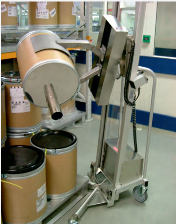
Rotating 180 degrees vertical to empty drums into hopper. Turning in the opposite direction, 130 degrees to dispense into weighing scales. Project nr DL03153.
