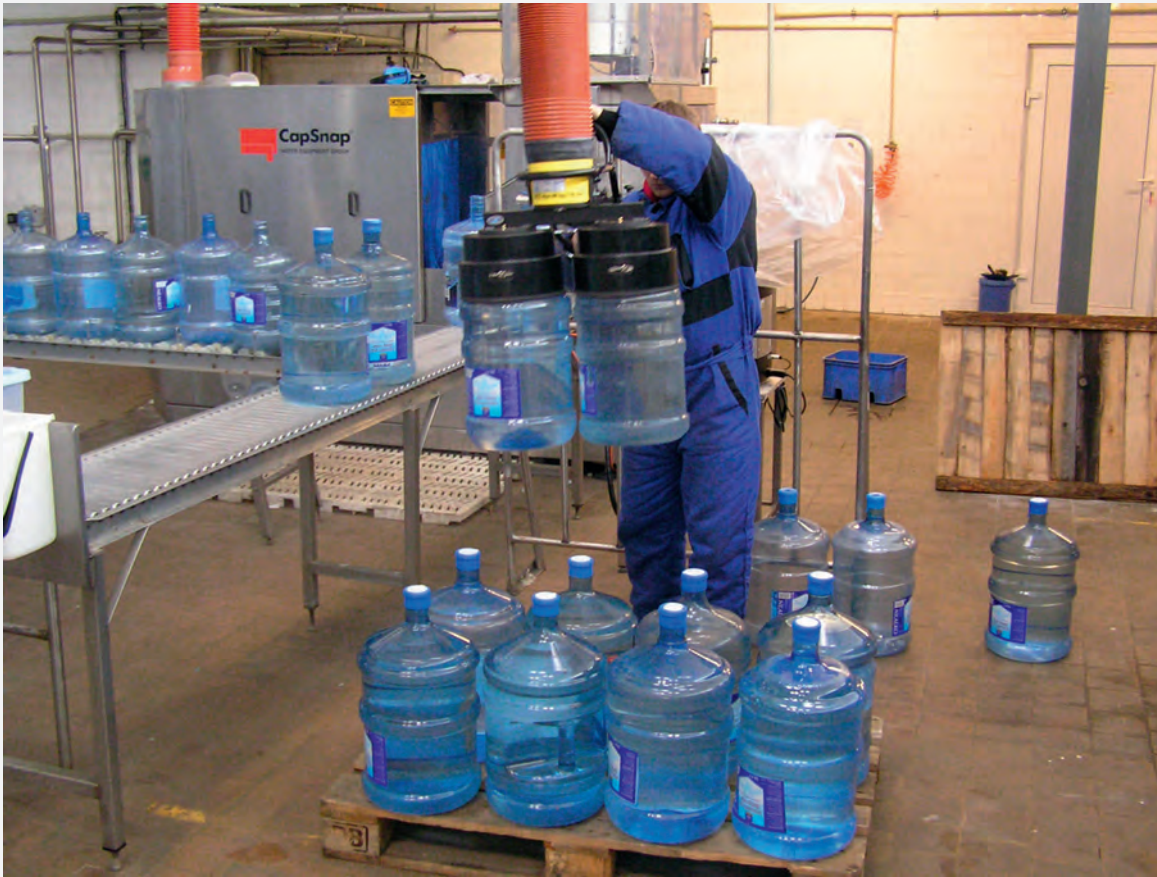
Two water dispensers at a time are lifted with this twin top lifter. Project nr 3340.
