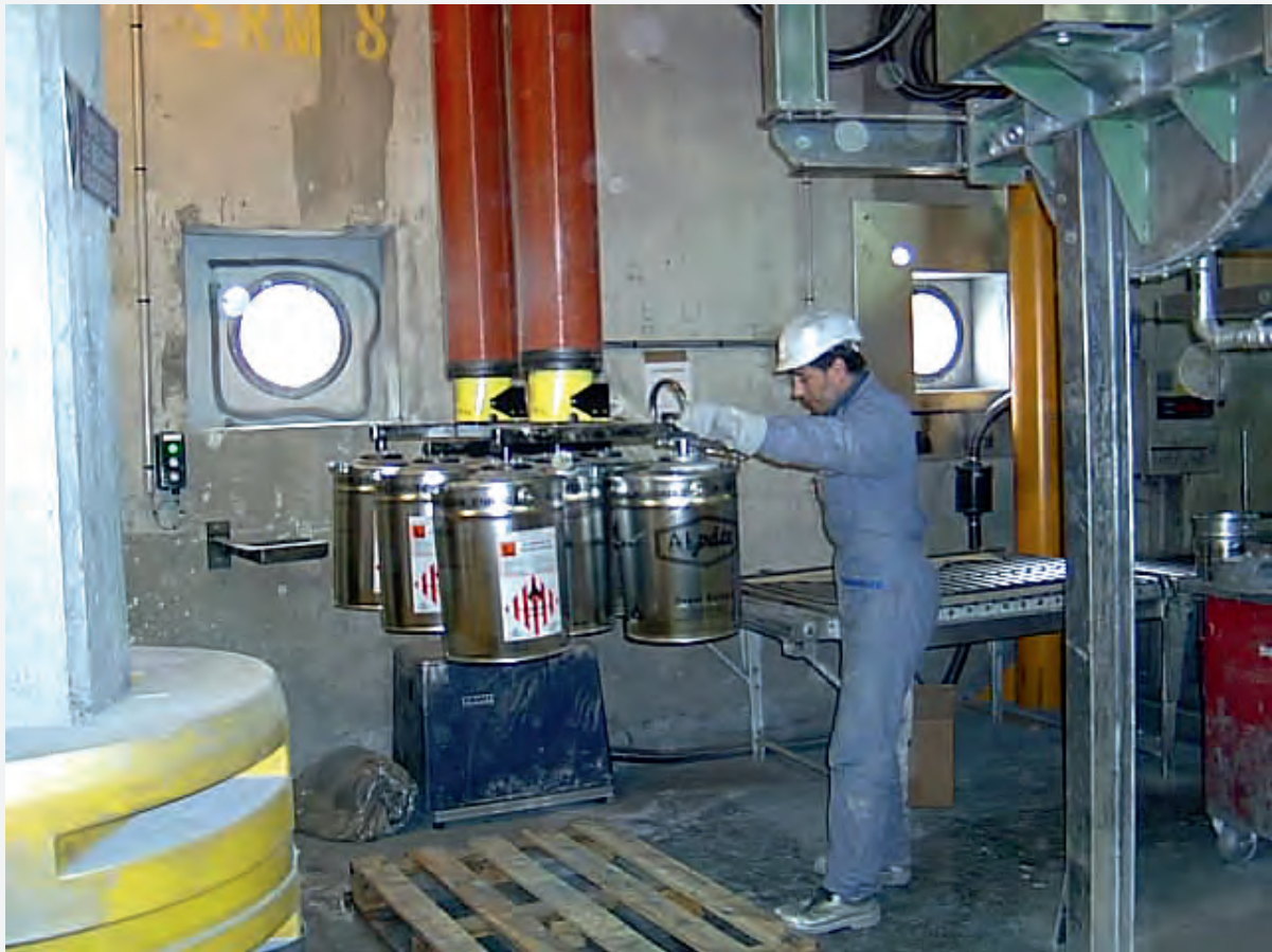
VM2200 with special suction foot to lift eight drums of chemical substance at a time. Suction foot project nr 2578.
