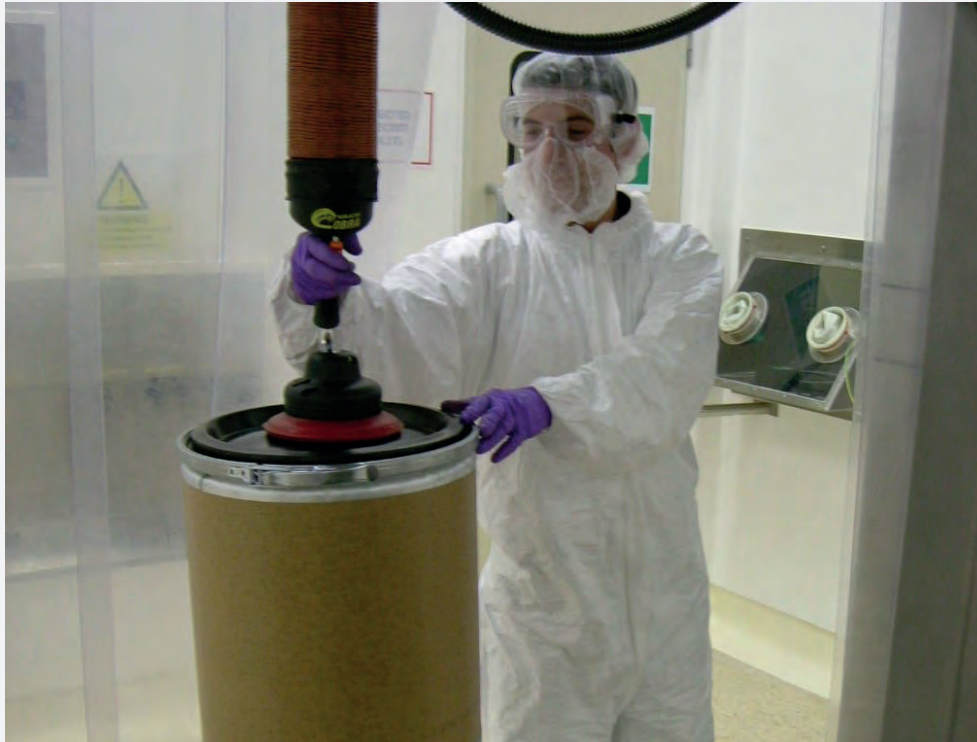
A stainless steel VacuCobra VC100, with max capacity 35 kg, is used to lift drums of tablets in cleanroom environment. The jib crane and column are also in stainless steel to meet the requirements of the client.
