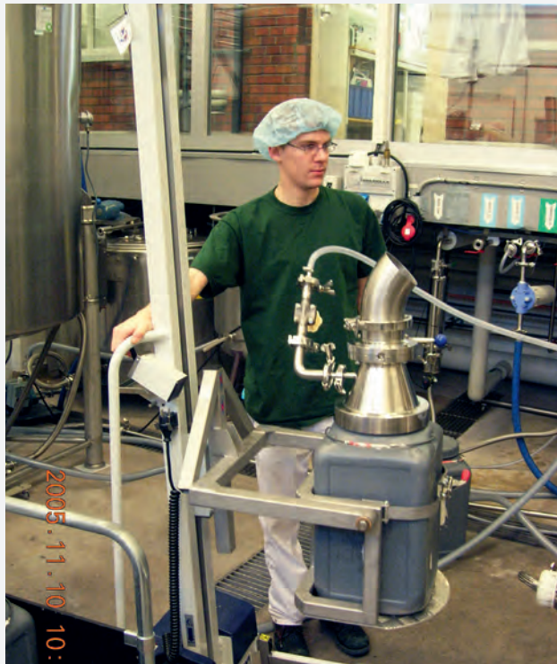
A drum turner on PRO70, this tool has max lifting capacity 40 kg. The liquid is moved to the production line and emptied into a container. Project nr DL02916.
