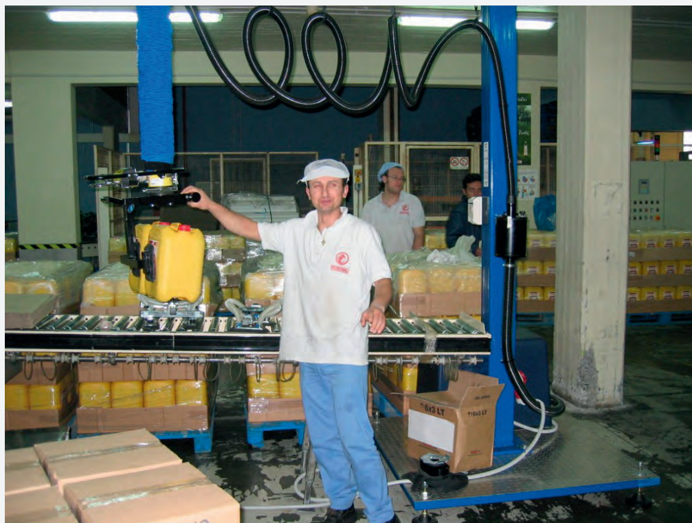
Two plastic containers lifted at the same time with a side lifter. VM100 max 30 kg. Project nr 2700.
