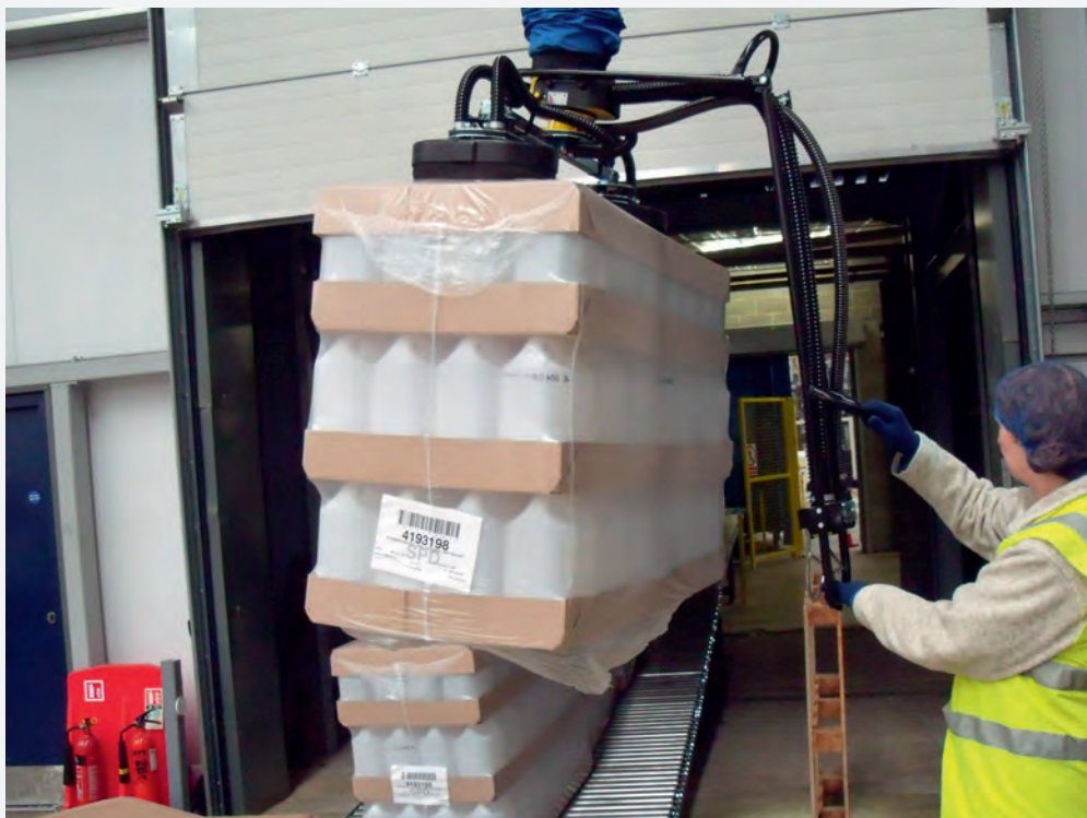
The extended, flexible handle makes it possible to lift HIGH up above shoulder height in an ergonomic fashion! Stacking at a height of 3200 mm, 3 batches on top of each other with a twin "sack-suction foot" on a yoke. This company manufactures plastic containers for all types of contents; oil, sprays etc.
