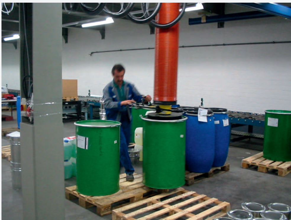
VM300 drum lifter. Suction foot project nr 1929.
