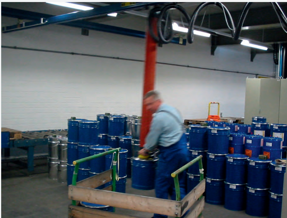
VM160 used to handle drums weighing appr 60 kg. The suction foot used in this application is standard, article nr 610230.
