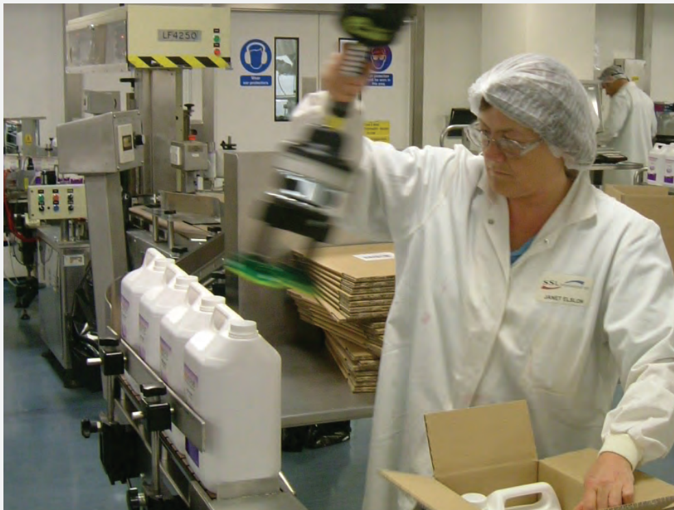
VacuCobra VC50 can lift objects weighing up to 8 kg with a suction foot measuring as little as 40 x 110 mm! This makes it suitable for high-frequency lifting in end-of-line, container packaging.
