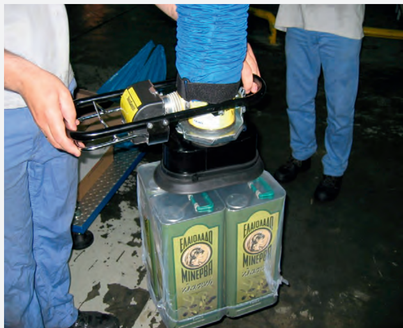
Shrinkwrapped containers of olive oil packed two-and-two, lifted with a VM100, max 30 kg and suction foot article nr 30300.
