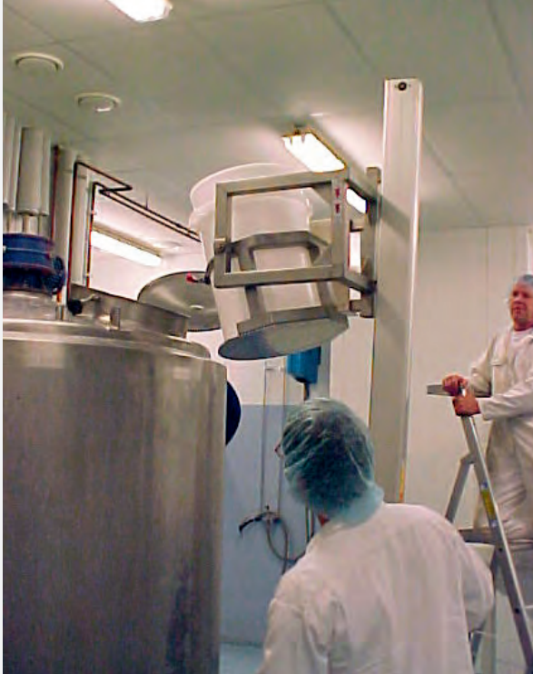
This electric lifter PRO120 has an extended mast and legs and is equipped with a cordless, 2-speed, remote control for lifting and rotating action. Project nr DL02762.
